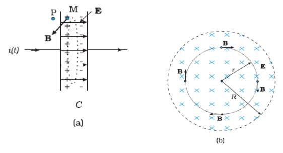
The electric field inside the plates of the capacitor is directed perpendicular to the plates. The magnetic field this gives rise to via the displacement current is along the perimeter of a circle parallel to the capacitor plates. So B and E are perpendicular in this case.
