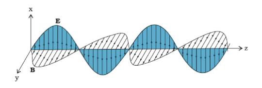
The above figure shows a typical example of a plane electromagnetic wave propagating along the *z* direction.
